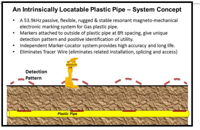
The program will be compatible with existing Plastic-Pipe Path locating products such as the EMS Locatable Tape and EMS Rope.
